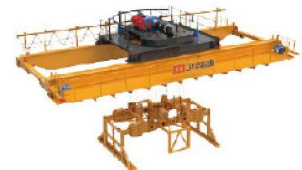
Cast Pipe Maintenance Crane
